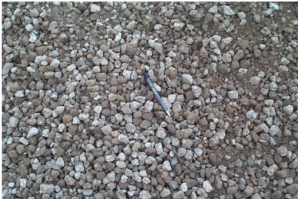
Figure 9. Finished recycled concrete aggregate.
