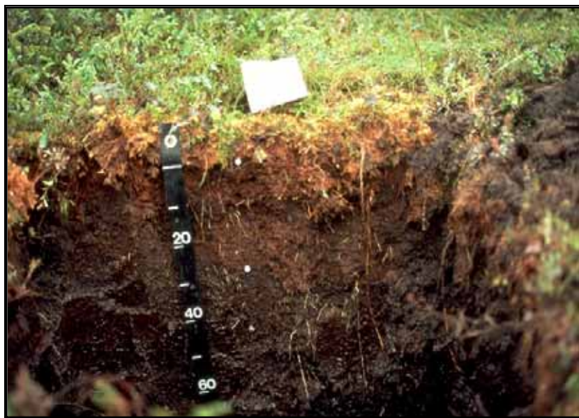
Figure 2. A saturated organic soil. In this profile, saturated organic material extends from the soil surface to a depth below 24 in. (60 cm). Scale is in centimeters.
