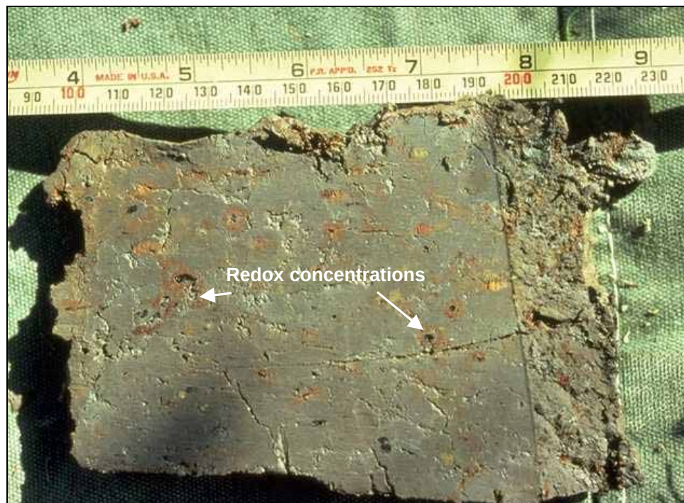
Figure 14. The matrix color meets the requirements of a gleyed matrix. Reddish-orange redox concentrations occur along root channels and other pores.
