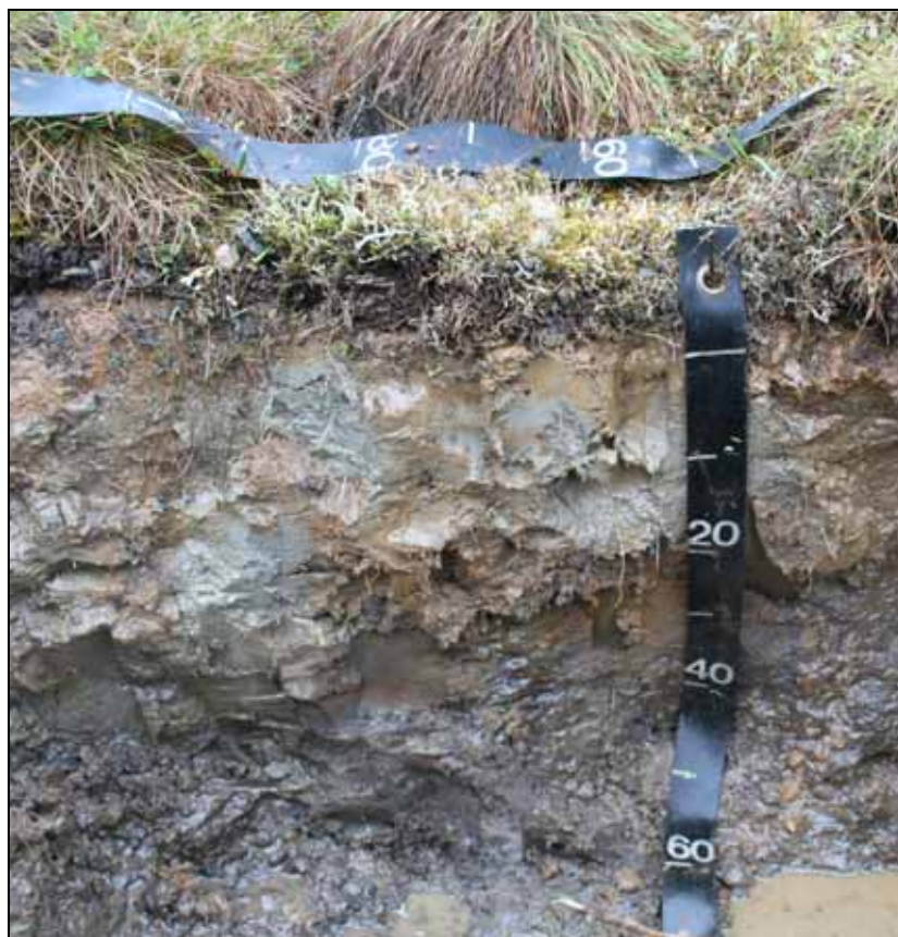
Figure 49. Water perched over permafrost at 16 in. (40 cm) and seasonal frost at 9 in. (22 cm) saturates this soil above 9 in. (22 cm). Note the reduced soil colors. Picture taken at the Toolik Lake Field Research Station, North Slope, on 18 July 2006. Scale in centimeters.
