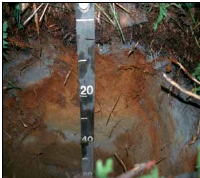
Figure 5. A well-drained Spodosol with strong E and Bh (spodic) horizons. Horizons have been broken and mixed by tree throw. Care is needed not to confuse these with redox depletions and redox concentrations caused by soil saturation and anaerobiosis.
