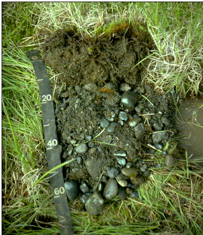
Figure 53. Low organic-matter content and coarse gravelly materials can make identification of hydric soil indicators difficult.
