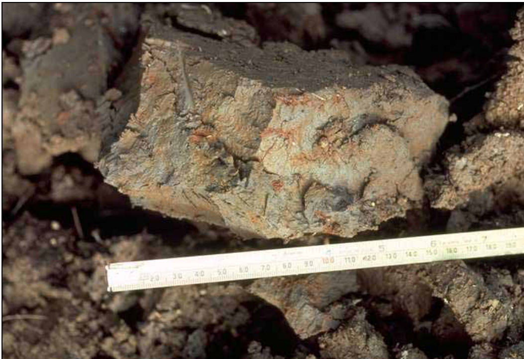
Figure 15. Gleyed matrix colors and reddish-orange iron concentrations. Concentrations are along root channels.
