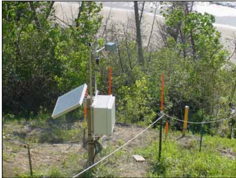
Figure 5. View from above of our site in a nearby control section of the bluff. Soil temperature, moisture, and resistivity instrument profiles in the bluff are marked by orange stakes, with solar panel, data logger, and web camera visible as a cluster in the foreground.
