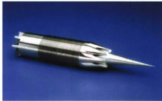
Figure 11. The gun-launched projectile design used eight scramjet wrapped around a cylindrical centerbody with fuel tank and delivery system.
