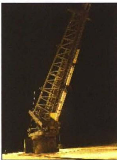
Figure 24. The payload vehicle and two-stage booster stack are rail mounted and launched along a suppressed ballistic trajectory.
