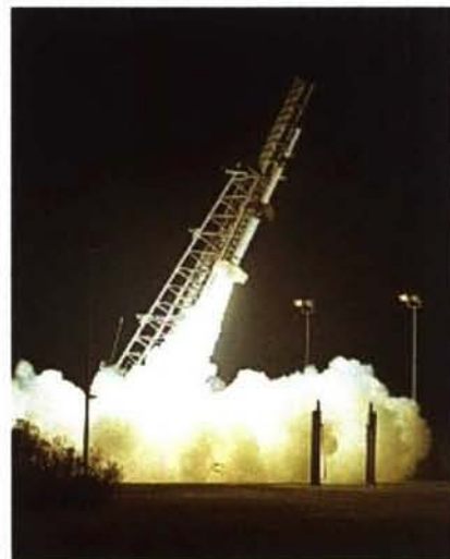
Figure 24. The payload vehicle and two-stage booster stack are rail mounted and launched along a suppressed ballistic trajectory.
