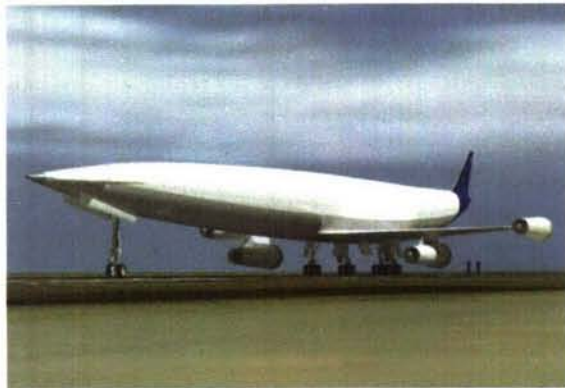
Fig. 12: Artist's impressions of LAPCAT A2. Left: Mach 5 hydrogen fuelled cruiser for 300 passengers with a MTOW of 400tons; right LAPCAT A2 compared with A380.
