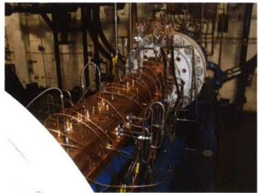
Figure 10. Initial configurations for a gun-launched scramjet featured a predominantly annular engine design that did not offer sufficient strength for high G loads. A direct connect test rig was used subsequently to develop a fully 3D engine configuration
