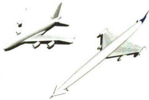
Fig. 12: Artist's impressions of LAPCAT A2. Left: Mach 5 hydrogen fuelled cruiser for 300 passengers with a MTOW of 400tons; right LAPCAT A2 compared with A380.
