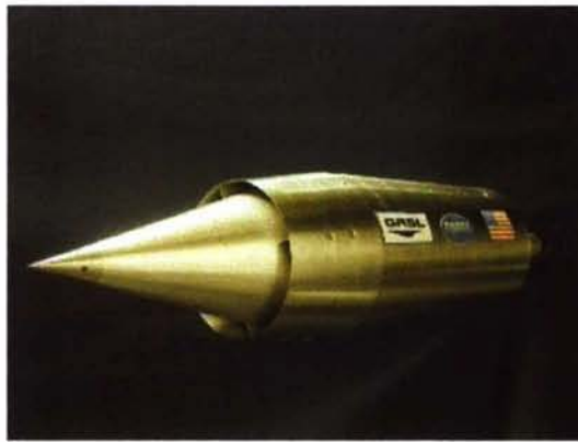
Figure 10. Initial configurations for a gun-launched scramjet featured a predominantly annular engine design that did not offer sufficient strength for high G loads. A direct connect test rig was used subsequently to develop a fully 3D engine configuration
