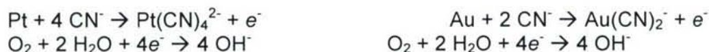
Figure 10. Electrochemical reactions responsible for the etching of platinum and gold by cyanide.
