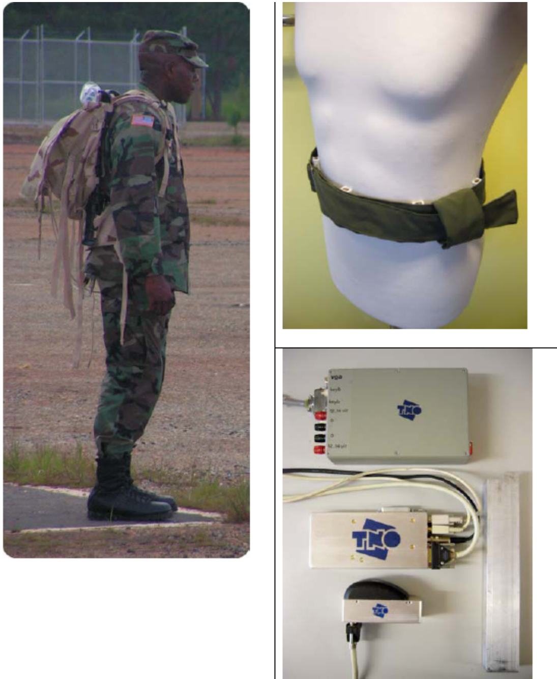
Figure 1. PTN, a torso-based tactile land navigation system. (Left: Soldier wearing PTN using a backpack to hold the system equipment. Top right: the tactile display [waist belt] with the tactors. Bottom right: the PTN system equipment [break-out box, microprocessor, sensor unit, battery unit].)
