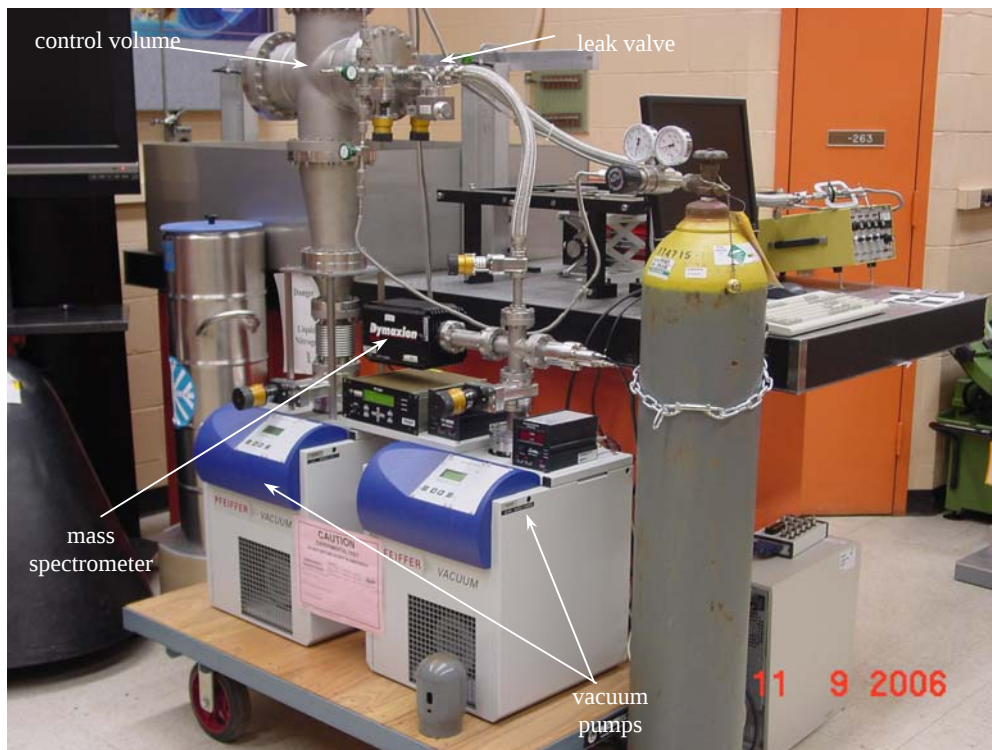
Figure 1: Permeability measurement apparatus
