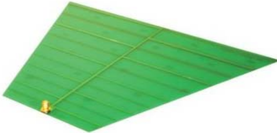
Figure 5. LPY41 log periodic antenna. (From Ramsey Electronics)
