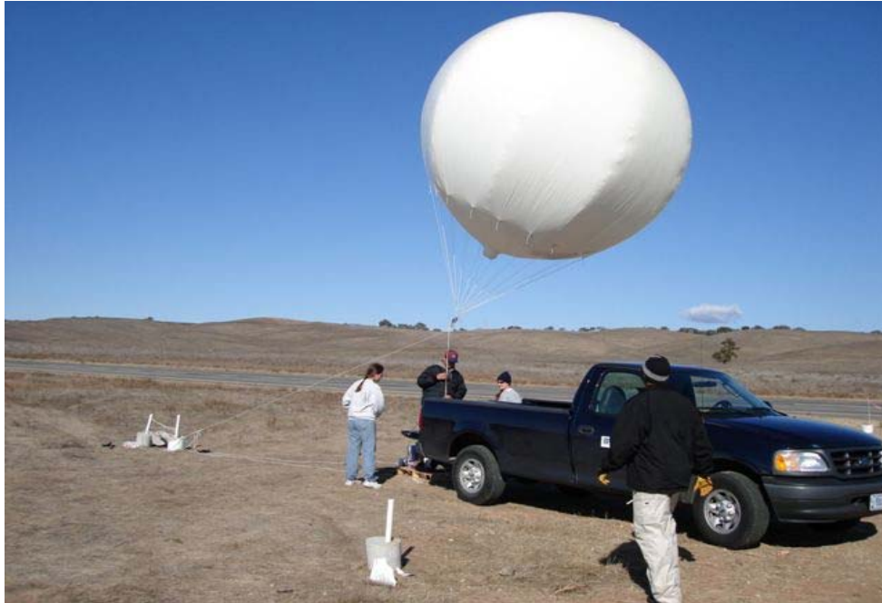
Figure 18. Attaching the repeater to a 10-foot-helium filled balloon.
