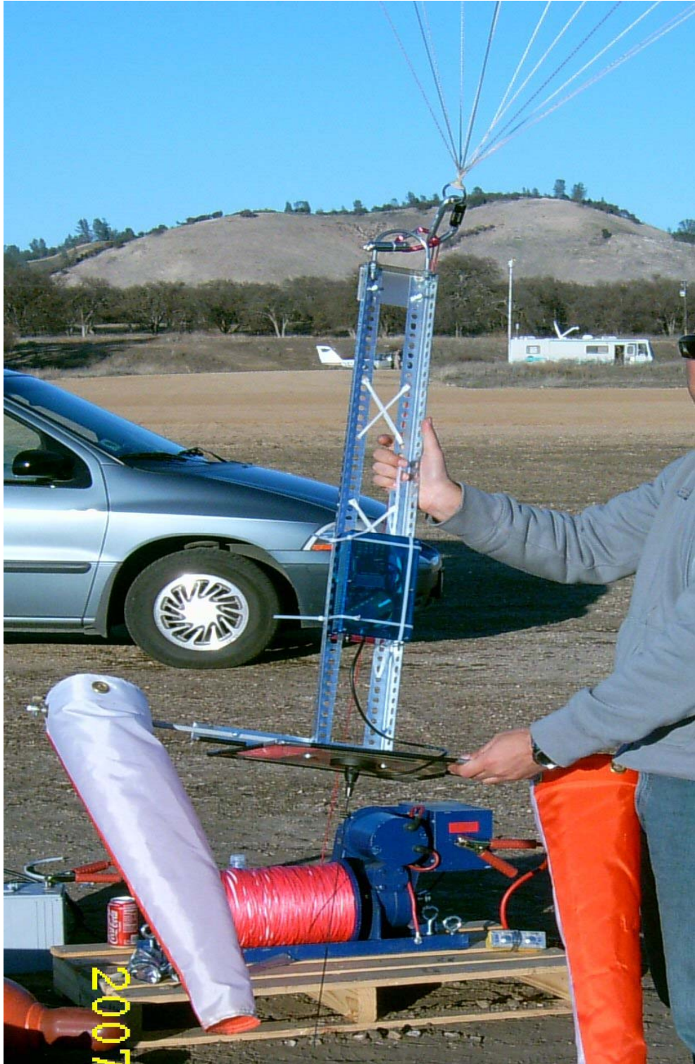
Figure 27. Payload consisting of ground plane antenna and repeater.
