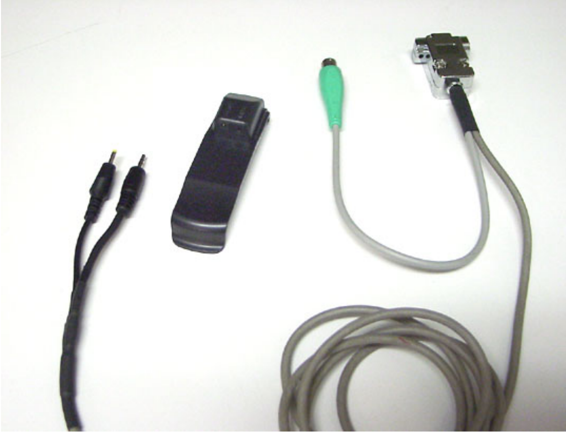
Figure 21. Power and data connections for the ForeTrex GPS receiver.
