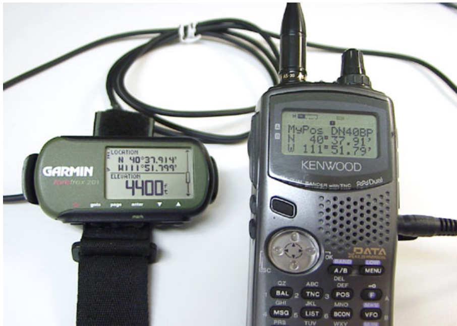
Figure 19. Foretrex 201 GARMIN "Personal Navigator" Wrist GPS.
