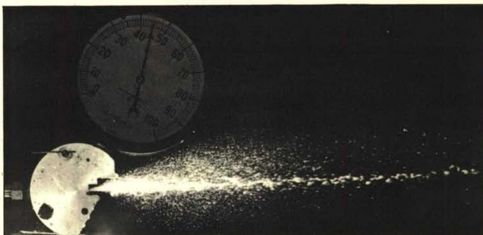
(A) INJECTION PRESSURE RAISED FROM ZERO TO TRANSITION POINT
