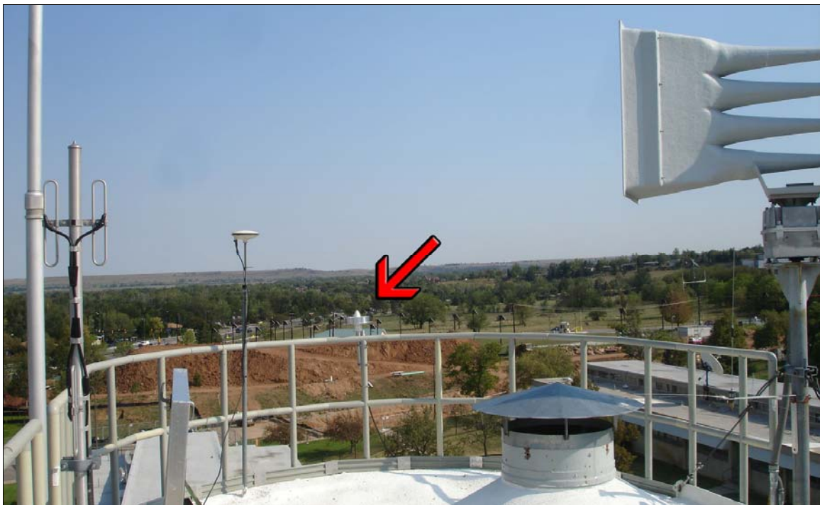
Figure 6. Antenna Site 1 (the arrow points to the choke ring antenna under test).
