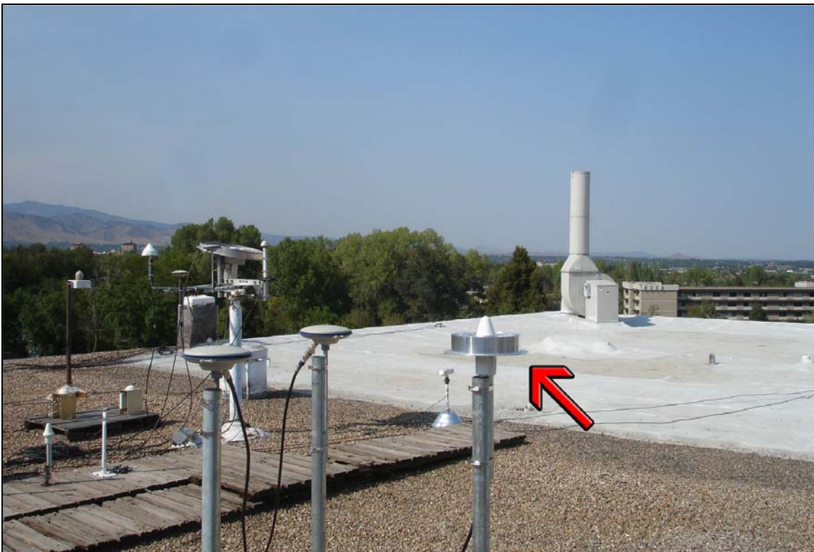
Figure 8. Antenna Site 3 (the arrow points to the choke ring antenna under test).
