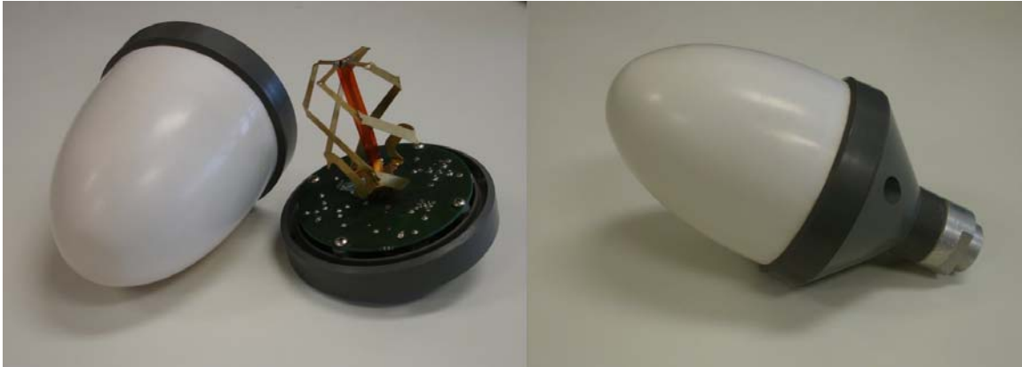
Figure 3. Quadrifilar helix antenna with radome removed (left) and with radome attached (right).
