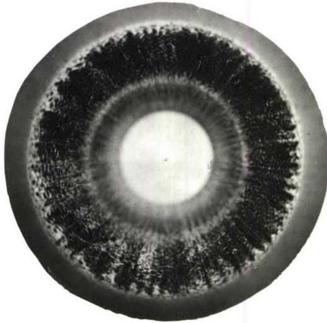
FIG. 6. Barrel L/112. Ex M.E.L.F. Fired 1228 bombs obtured P.V.C. rings. Breech end view.
