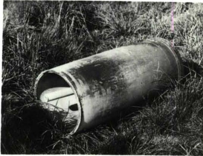
TYPICAL VIEW OF "100 lb." VESSEL, THE END OF WHICH BLEW OFF BEFORE THE BURSTING STRENGTH OF THE TUBE WAS REACHED. CONSTRUCTION OF VESSEL AS SHOWN IN FIG. 4. USED WITH UNCURED PROPELLANT. FIG. 5.
