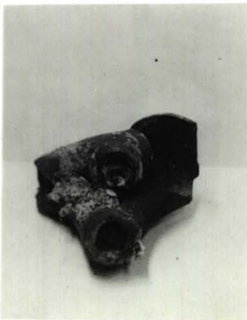
SHOT No. 3. AMMONIUM PERCHLORATE MIXED FOR 5 MINUTES WITH OTHER CON- STITUENTS.
