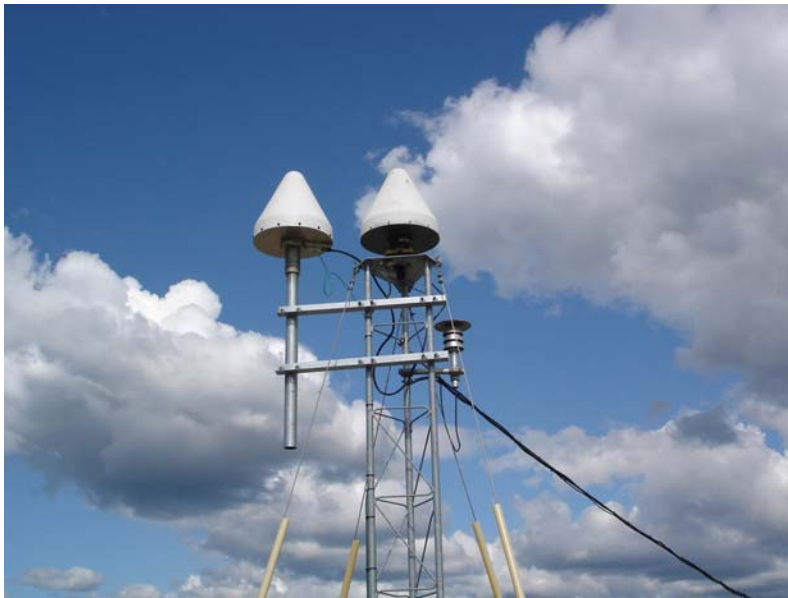
Figure 9. Dual antennas at the NGA monitor station in Alaska to be used for phase measurement cycle-slip detection/correction testing.
