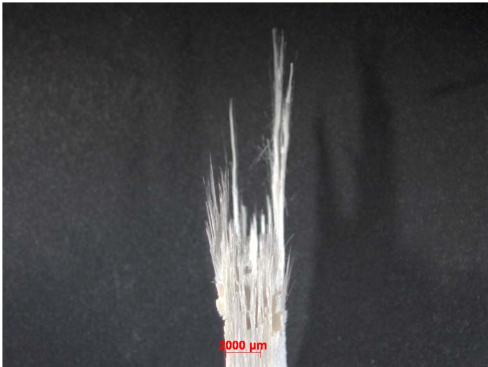
Figure 62. Fracture surface of N720/A specimen tested with cyclic creep-recovery with 1 hour hold times at 100 MPa in air at 1200 °C.
