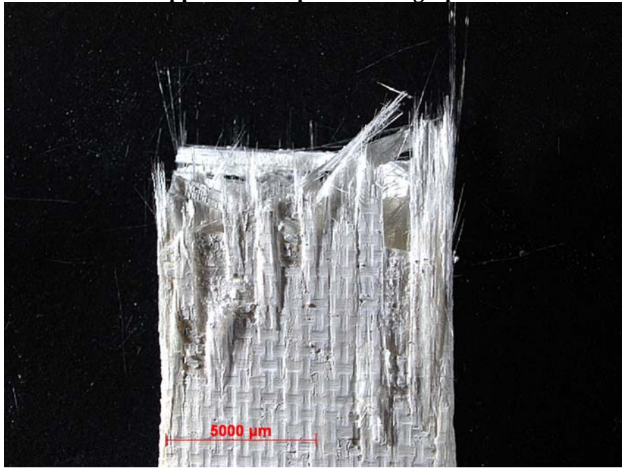
Figure 53. Fracture surface of N720/A specimen tested with cyclic creep-recovery with 30 hour hold times at 100 MPa in air at 1200 °C.
