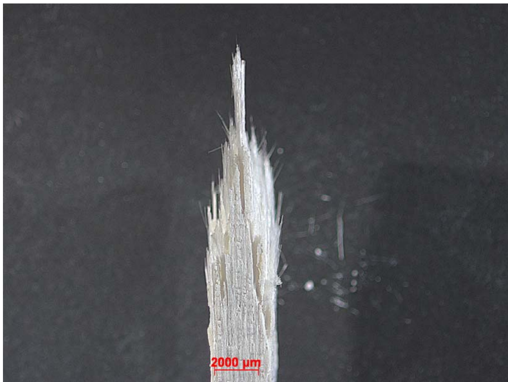
Figure 75. Fracture surface of N720/A specimen tested with cyclic creep-recovery with 1 hour hold times at 100 MPa in steam at 1200 °C.
