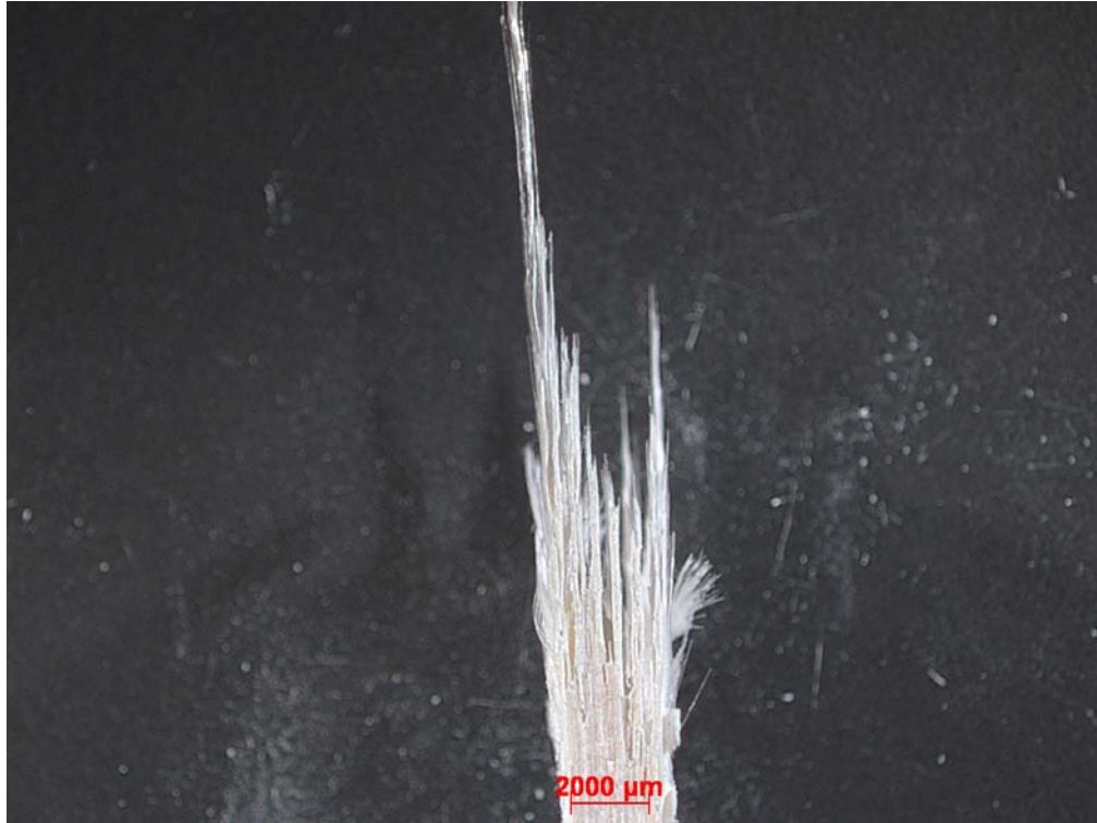
Figure 69. Fracture surface of N720/A specimen tested with cyclic creep-recovery with 1 hour hold times at 125 MPa in air at 1200 °C.
