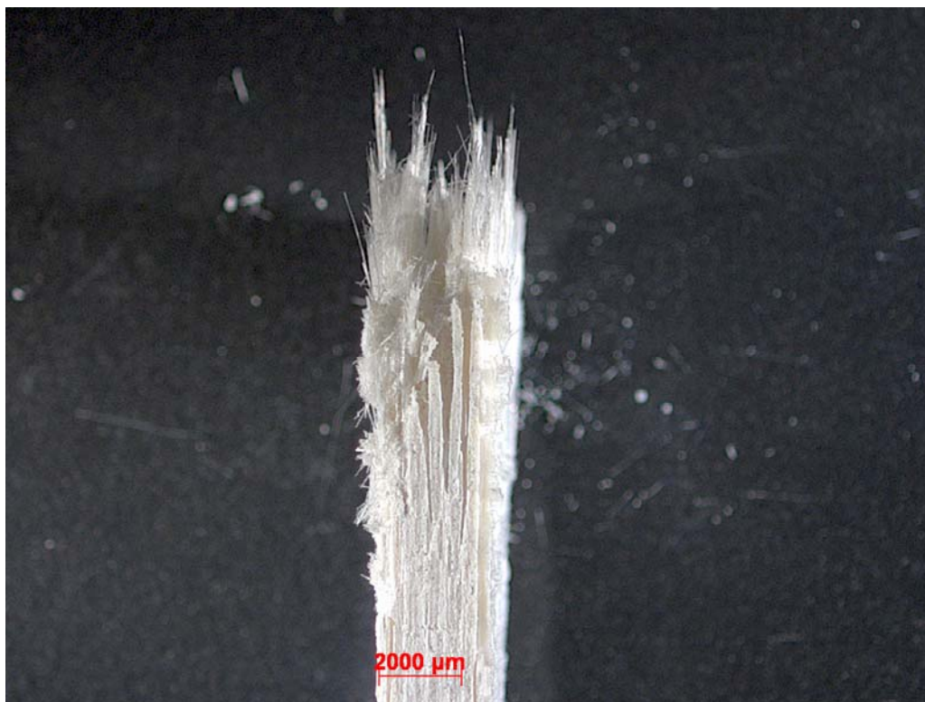
Figure 64. Fracture surface of N720/A specimen tested with cyclic creep-recovery with 1 hour hold times at 100 MPa in air at 1200 °C.
