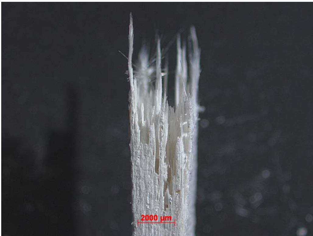
Figure 72. Fracture surface of N720/A specimen tested with cyclic creep-recovery with 1 hour hold times at 100 MPa in steam at 1200 °C.
