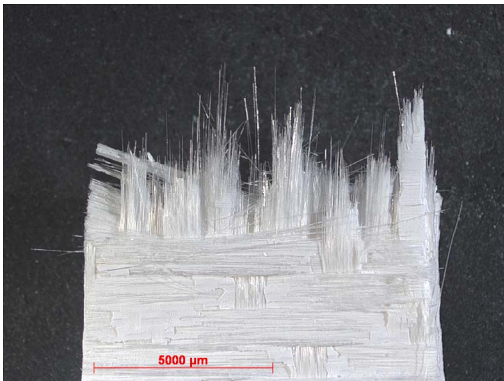
Figure 78. Fracture surface of N720/A specimen tested with cyclic creep-recovery with 1 hour hold times at 100 MPa in steam at 1200 °C, possible kinking.
