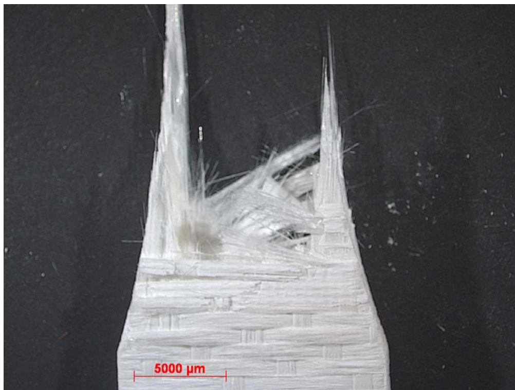
Figure 67. Fracture surface of N720/A specimen tested with cyclic creep-recovery with 1 hour hold times at 125 MPa in air at 1200 °C.
