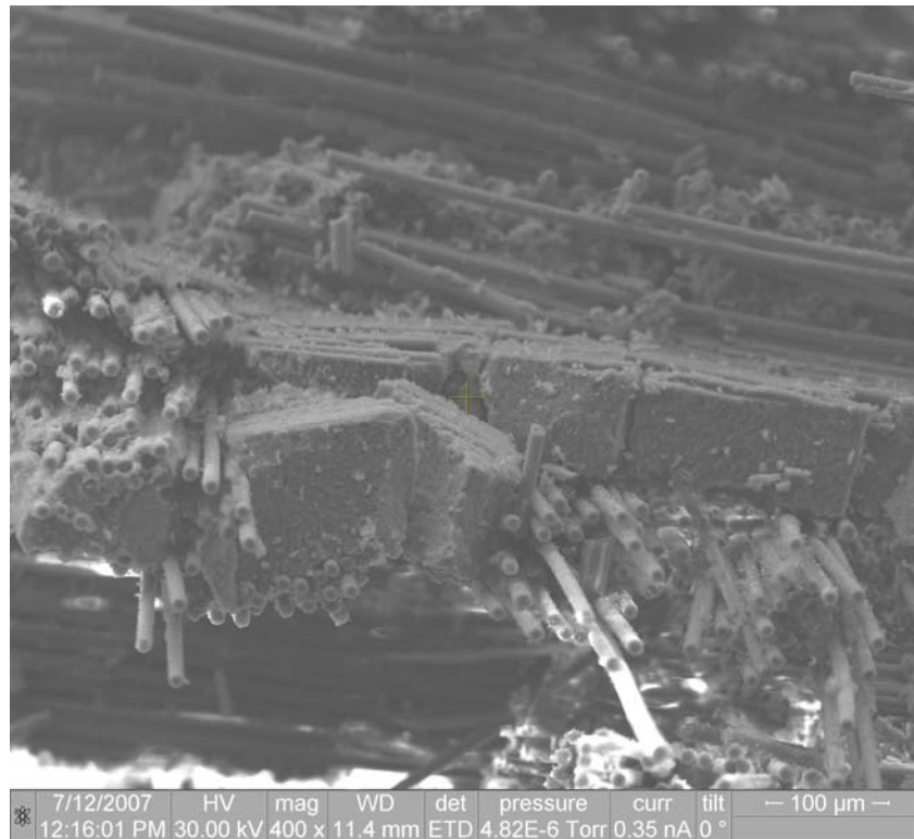
Figure 151. Fracture surface of N720/A specimen tested with cyclic creep-recovery with 1 hour hold times at 100 MPa in steam at 1200 °C, possible kinking.
