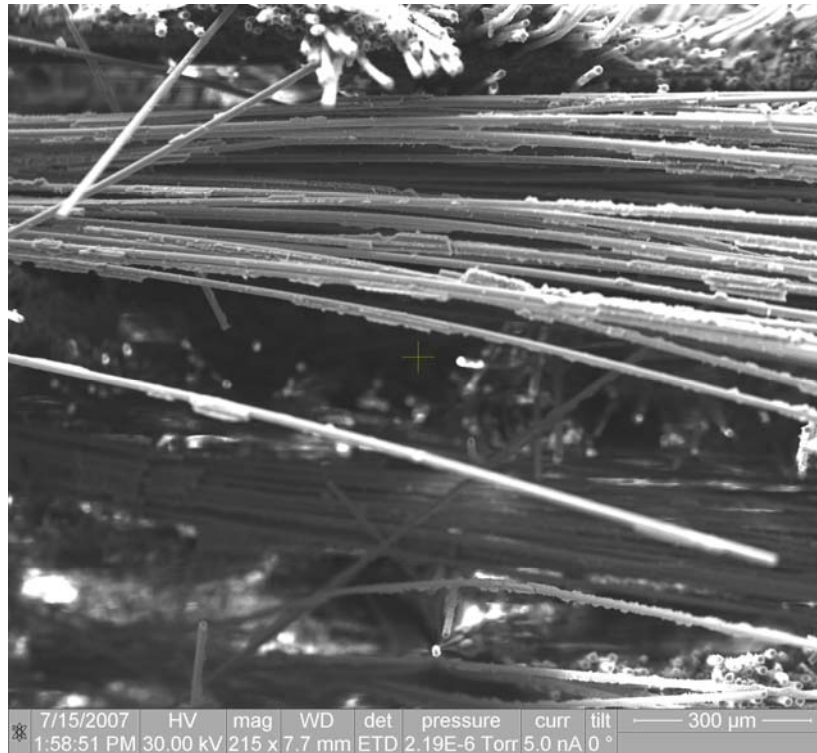
Figure 115. Fracture surface of N720/A specimen tested with cyclic creep-recovery with 1 hour hold times at 100 MPa in air at 1200 °C.
