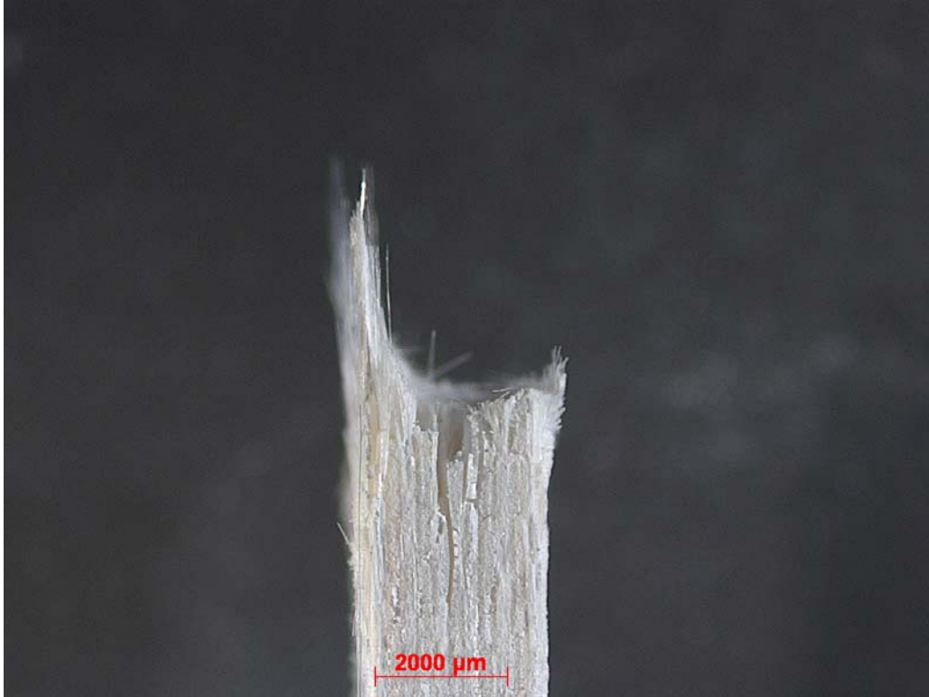
Figure 79. Fracture surface of N720/A specimen tested with cyclic creep-recovery with 1 hour hold times at 100 MPa in steam at 1200 °C, possible kinking.
