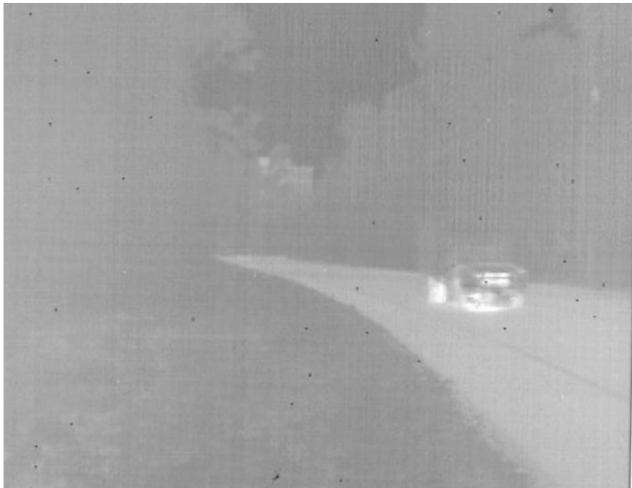
Figure 62. Typical IR image showing lack of background detail.
