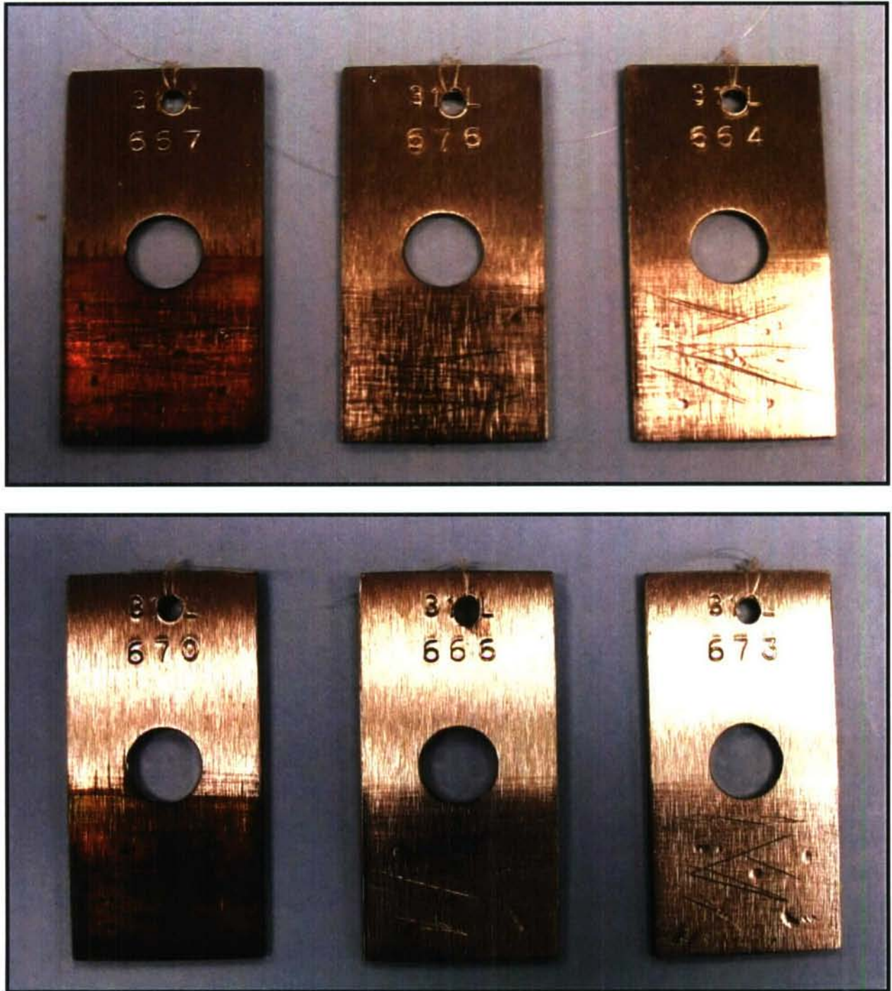
Figure 14. Example Photographs of the Soak and Soak/Brush Cleaning Scenarios for Rough Finish Treatment. The top panel is the soak scenario and the bottom panel is the soak/brush scenario. Deionized water is on the left, peracetic acid is the middle, and \text{HPO}_2^{\text{TM}} reagent is on the right.
