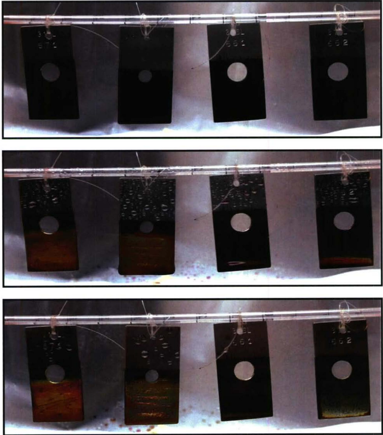
Figure 15. Example Photographs of the Spray Cleaning Scenario Using Deionized Water. The top panel is the contaminated coupons, the middle panel is the coupons after reagent, and the bottom panel is the coupons after water rinse and air drying for 15 min.
