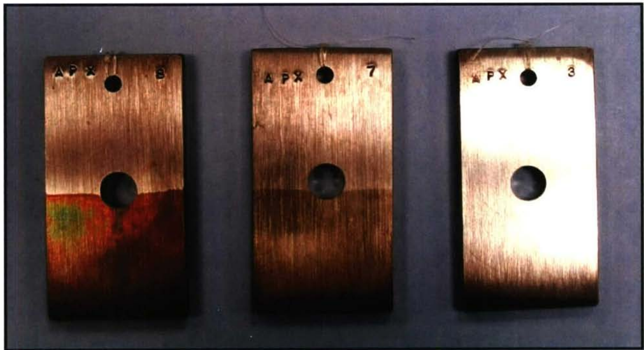
Figure 13. Example Photographs of the Soak and Soak/Brush Cleaning Scenarios for Smooth Finish Treatment. The top panel is the soak scenario and the bottom panel is the soak/brush scenario. Deionized water is on the left, peracetic acid is the middle, and \text{HPO}_2^{\text{TM}} reagent is on the right.
