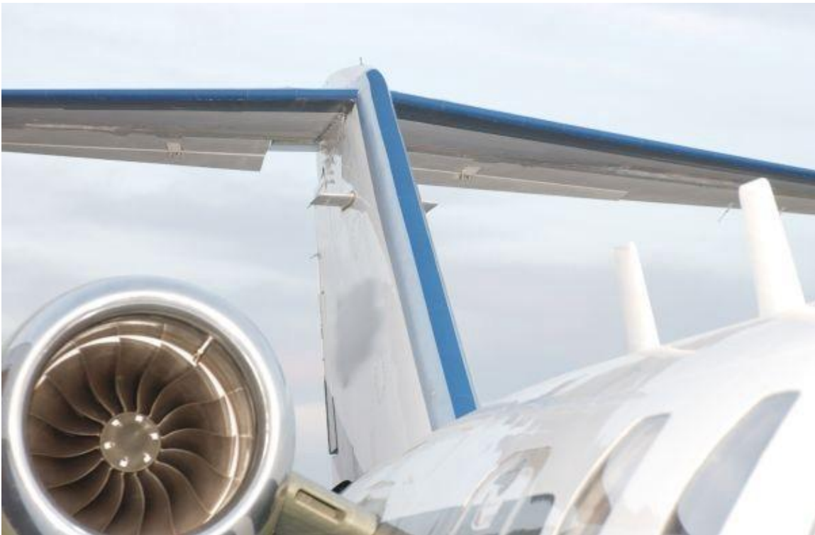
Figure 71. - 40 grit sandpaper (darker blue areas) on horizontal and vertical tail leading edges to simulate inter-cycle ice.
