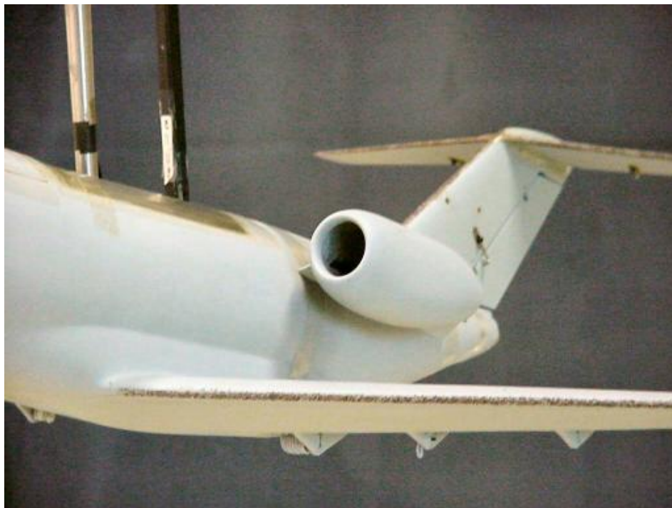
Figure 14. – Pre-Activation Ice representation on 1/12-scale model.
