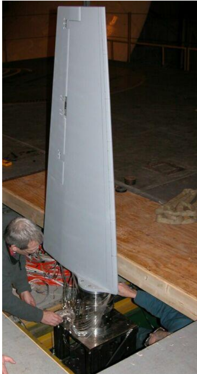
Figure 4. – Photograph of the installation of the 5/12-scale wing panel in the LFSWT showing the spacer mounted under the TDT-05S balance.
