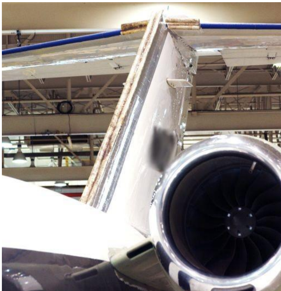
Figure 74. - Ice shapes used on tail surfaces during run-back and failure ice conditions.
