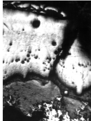
Fig. 2 – Spalling of the secondary structure, x120
