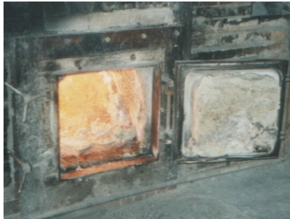
Dr. 2. Refractory concrete BRAB30И15κ* with oxide-ceramic covering «M-1*» after 6 months of operation, february 2004.
