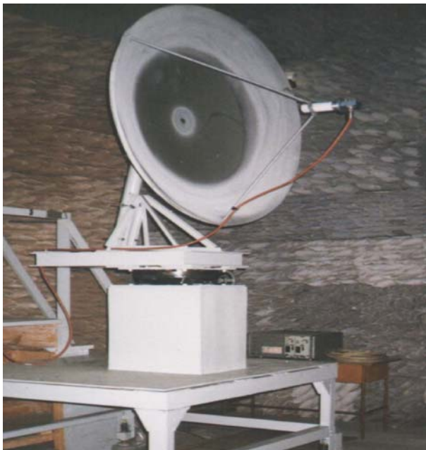
Fig. 2. Parabolic aerial with functional coatings
