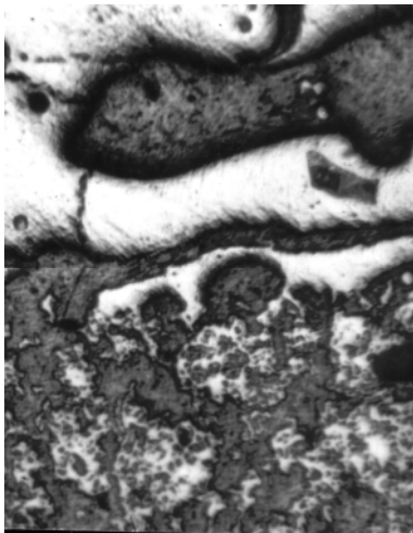
Fig. 1 – Failure secondary structure, x120
