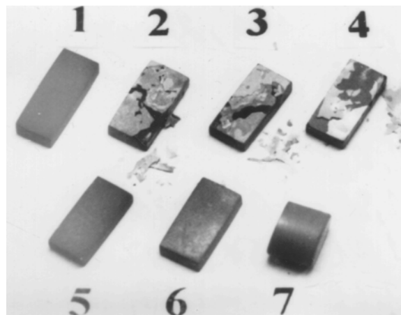
Fig. 1. Photograph of the titanium alloys samples after oxidation at 800 °C, 20 h:
