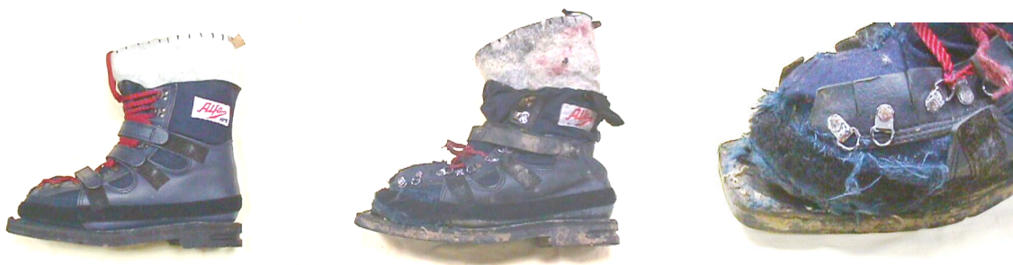
Figure 2. Photographs showing the FS in a new, unused condition (left) and after the 109 day Arctic Ocean ski trek (center and right).
