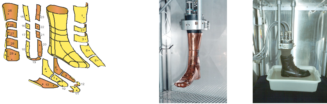
Figure 1. Diagram showing regional sections of the TFM (left) and photographs showing the TFM bare (center) and during typical military footwear testing (right).
