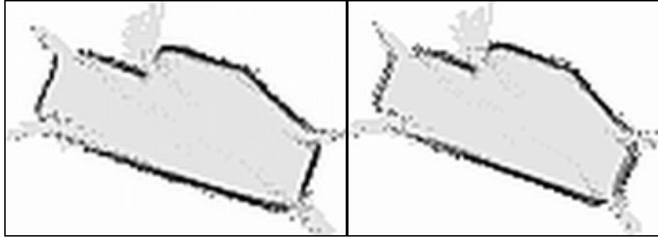
Figure 20. Maps generated using a good motion model (left) versus an initially skewed model with learning (right). The close similarity demonstrates how the robot has learned the correct motion model.
