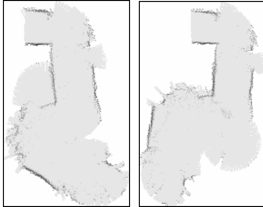
Figure 28. Maps generated by non-learning SLAM (left) and learning SLAM (right) given an incorrect motion model for the operating surface.
