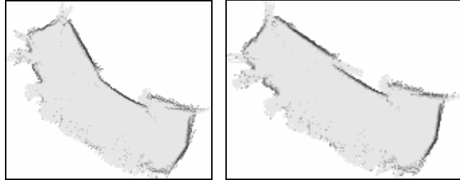
Figure 29. Maps generated by non-learning SLAM (left) and learning SLAM (right) using the motion model for one robot as the input for a completely different robot.
