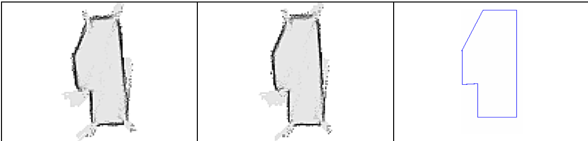
Figure 19. Maps generated by non-learning SLAM (left) and learning SLAM (center) applications when input was the measured motion model. Each pixel in the map represents approximately a 4x4 cm segment of floor space with the entire room measuring 133x305 cm. Note that maps are nearly identical and accurately represent the room's floor plan (right).
