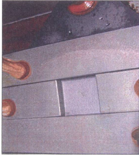
Water Jet Milling Simple Masking Setup
