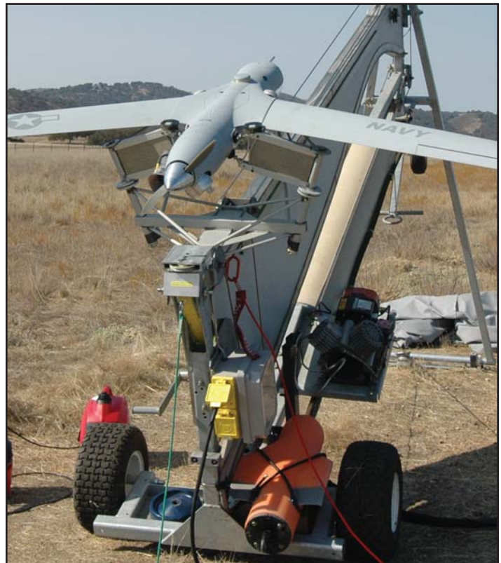
A Scan Eagle unmanned aerial vehicle sits on a launch sled during USSOCOM sponsored Tactical Network Topography 07-1 experiment at Camp Roberts, Calif.
