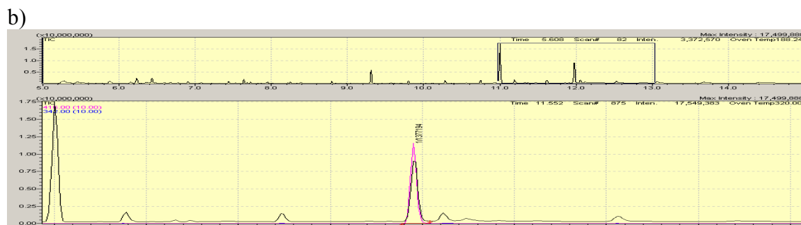
Figure 2.5 GC-MS spectra for standard [Estradiol] =3200 pg/ml a) underivatized and b) derivatized.
