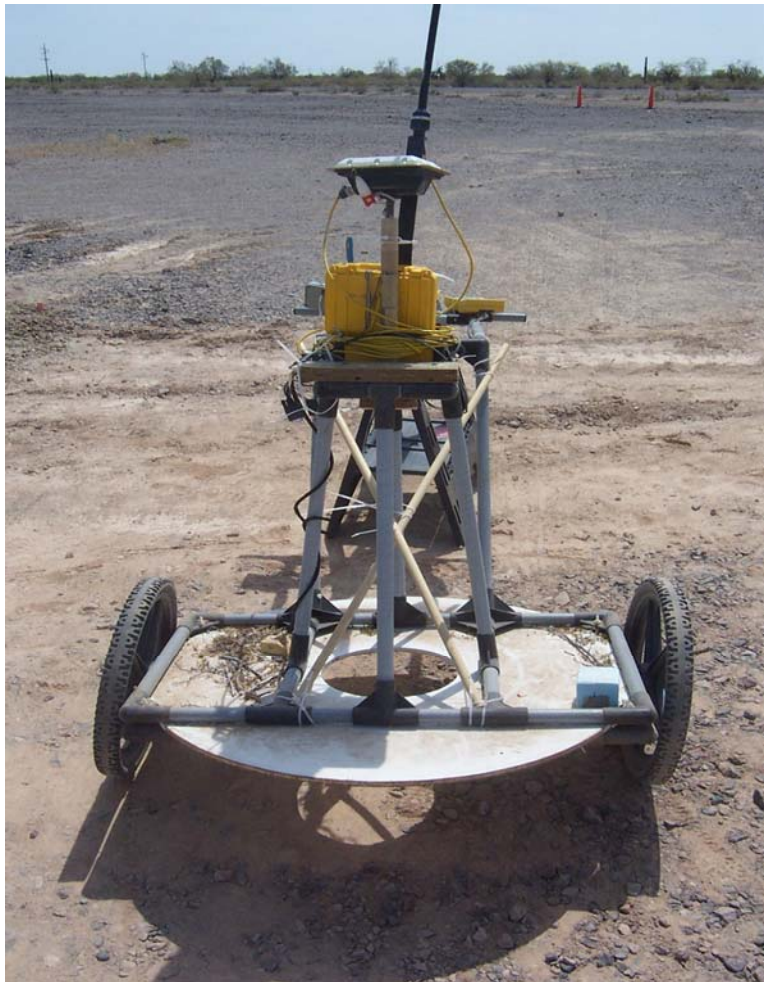
Figure 6. The GEM-3-E cart system with controller and GPS.
