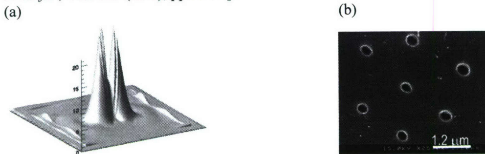
Fig. 3 (a) Numerical simulation using finite difference time domain method shows strong laser intensity enhancement due to the nanosphere; (b) experimental demonstration shows a 200-nm hole array was produced on glass.
