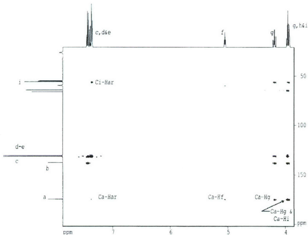
Figure 6. ^1\text{H} - ^{13}\text{C} HMBC Sub-Spectrum of the Unidentified Powder Dissolved in \text{D}_2\text{O} with the Corresponding Regions of the ^1\text{H} and ^{13}\text{C}\{^1\text{H}\} Spectra. Long-range correlations demonstrating the connectivities of specific chemical groups in the molecule are labeled.
