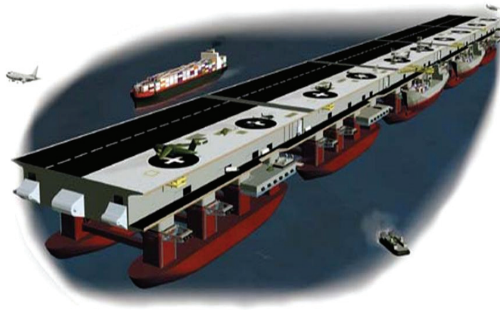
Figure 4: Joint Mobile Offshore Platform 80
