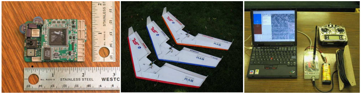
Figure 12. Hardware platform used to obtain experimental results. The first frame shows the Kestrel autopilot designed at BYU. The second frame shows airframes similar to those used in this study. The third frame shows the ground station components for our testbed.
