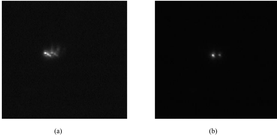
Figure 4: Single frame image of the binary star \beta Delphini. (a) open loop frame, (b) closed loop frame.
