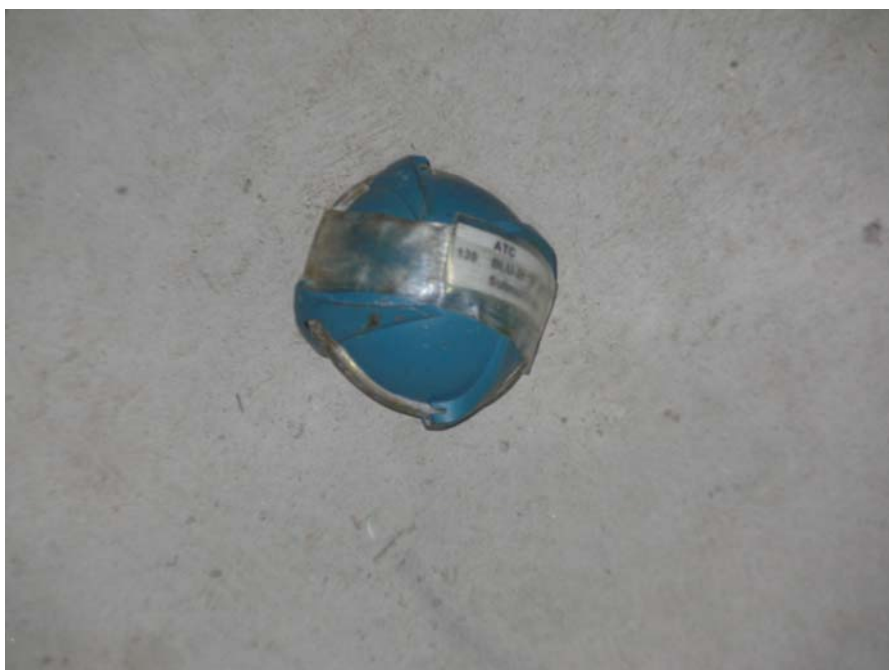
Figure 2.1-7. Bomb, BLU 26, inert submunition.
