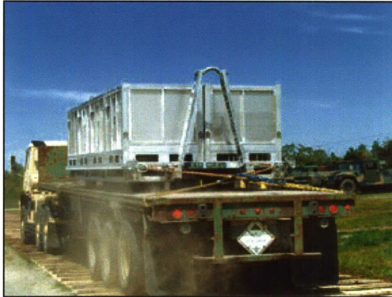
Photo 14. Washboard Course Testing of the JMIP
