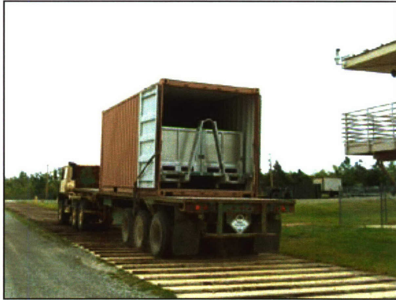
Photo 4. Washboard Course Testing of the JMIP
