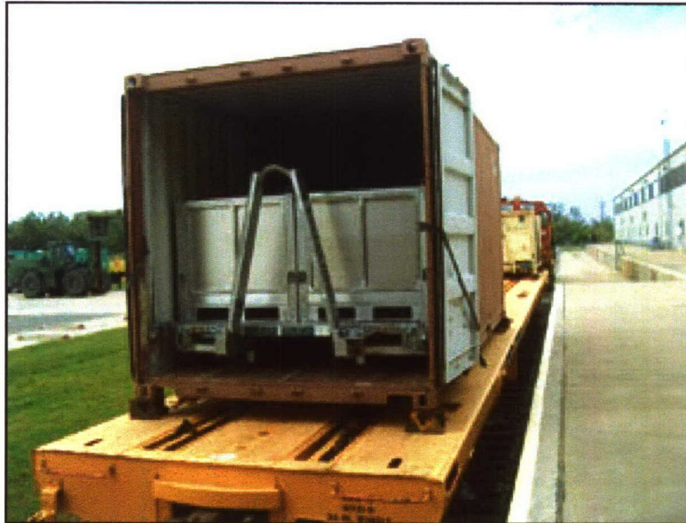
Photo 2. Rail Impact Testing of the JMIP (Prior to Testing)
