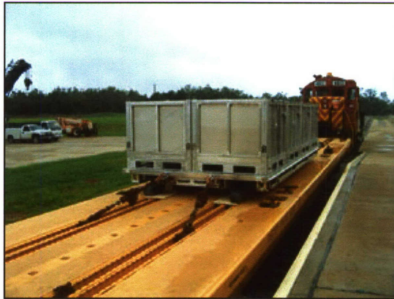
Photo 15. Rail Impact Testing of the JMIP (Prior to Testing)
