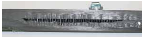
Figure 7: Photograph of 0.125 inch Stubble Specimen Without 2 nd Ultrasonic Step
