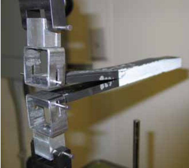
Figure 6: Photograph of DCB Specimen in Pin-Loaded Fixture
