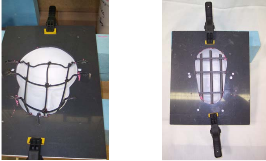
Figure 3. Mask form holder constructed from PVC
