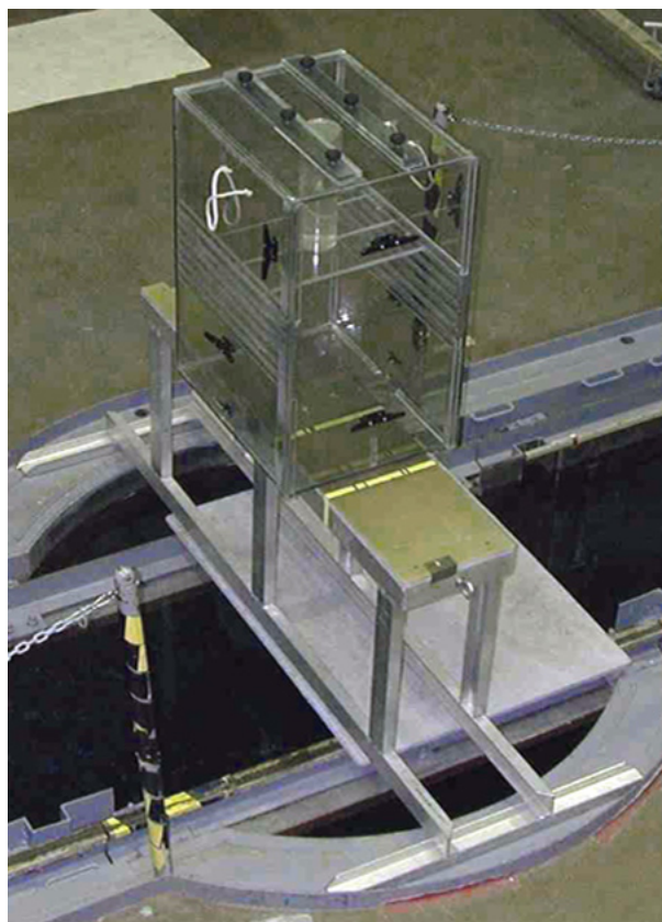
Figure 6. A high-angle view of the acrylic plastic NHP-restraint box centered on the table in the AFRRI ^{60}\text{Co} whole-body irradiator. The restrainer is secured to the table during animal irradiation with elastic straps. The table is immobilized by aluminum beams, secured to the bottom of the table, that contact the arcs located on the top of the pool. A water-filled PMMA cylinder used for dosimetry is located between the white ropes used for carrying the restraint box.
