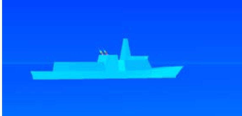
Figure 2.11 Typical output from ShipIR (adapted from Ref. 22)
