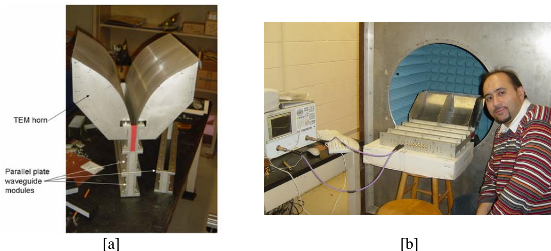
Figure 6: Measuring infinite x 8 DmBAVA array with TEM horn “load”. [a] Parallel plate waveguide simulator with TEM horn extension. [b] The final measurement setup: mini-range chamber, parallel plate waveguide simulator with TEM horn, 2Ports HP Power Network Analyzer (PNA).
