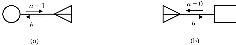
Fig. 1. The definition of (a) an ideal amplitude source (circle) connected to a Tx antenna by a feed line; and (b) an ideal amplitude meter (square) connected to an Rx antenna via a feed line. Both meters are matched to the feed line (antenna impedances are not necessarily matched to the feed line).
