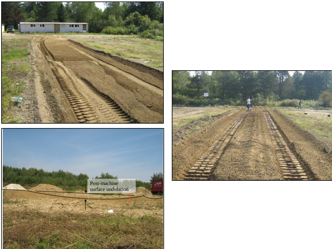
Figure 24. Terrain After Passage Of MineWolf Without (Left) and With (Right) Automatic Depth Control
