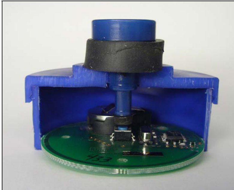
Figure A-4 Cut-away View of WORM Test Target
