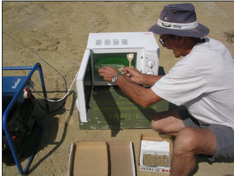
Figure A-3. Soil Drying Using a Microwave
