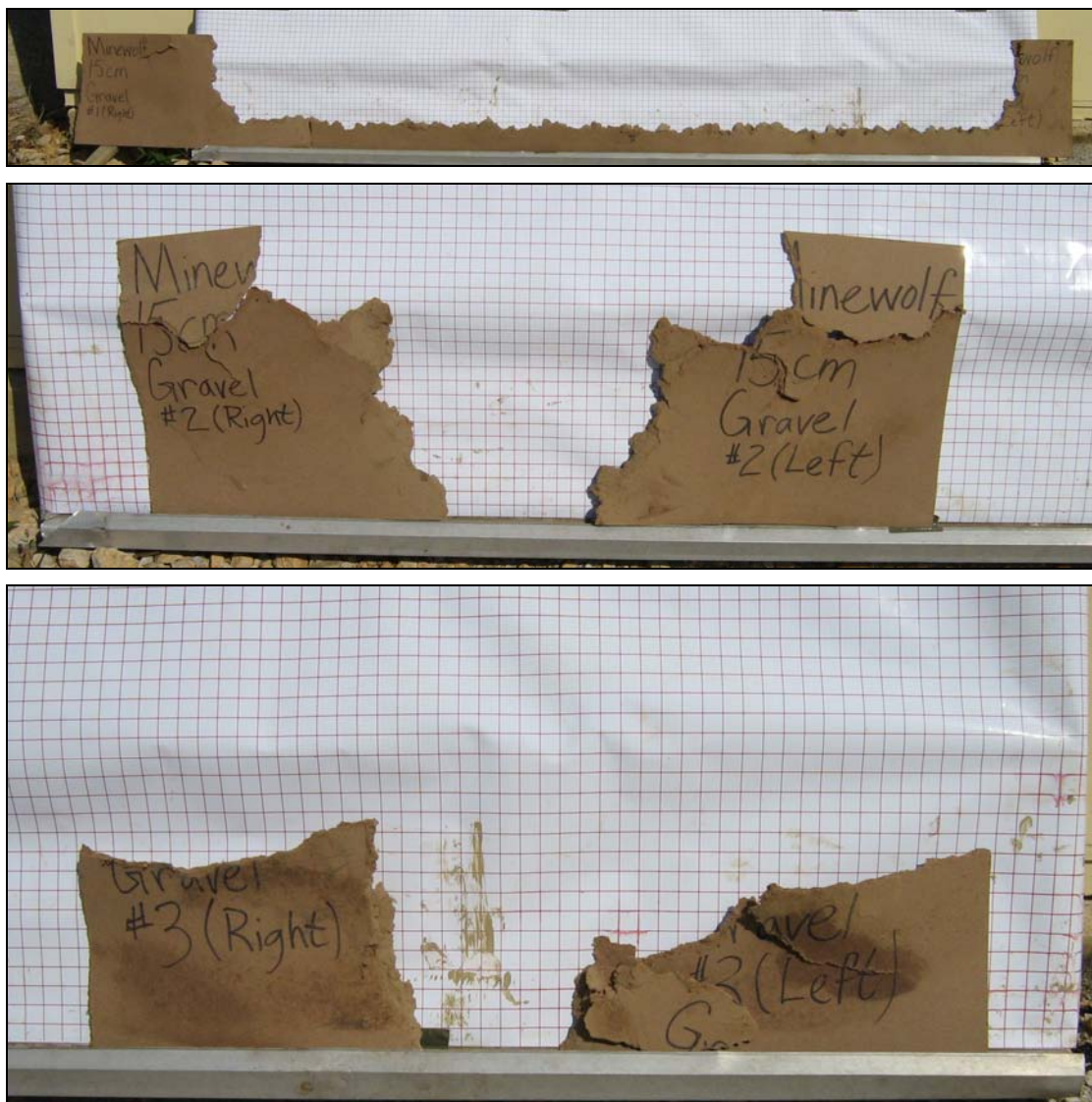
Figure 20. Depth of Penetration in Gravel with mines at 15 cm DOB
