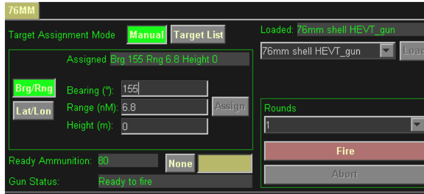
Figure 5: The Gun Controller Interface for Manually Entering Target Information
