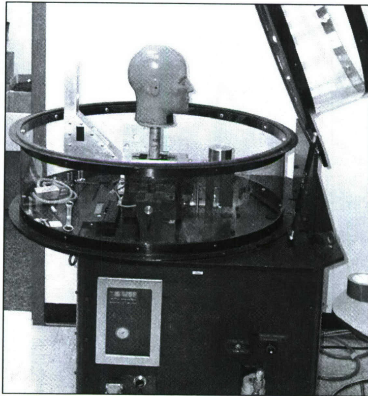
Figure 7. KSR330-60 Mass properties instrument.
