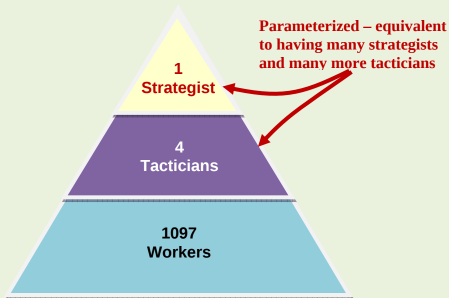
Figure 1: The architecture of the Cyc inference engine. This can also serve as a “harness” for other reasoning systems, which can be “published” as new Workers (proxies who just call the external reasoning system). These proxies can be characterized the same as the other 1097 Workers, so they can be called on when and as appropriate, to tackle sub-problems they would be good at, and can recursively re-broadcast sub-sub-problems back to the overall assemblage of modules – i.e., to the overall inference engine, hence they might end up being called on multiple times in the course of solving a single problem, with different sub-problems.
