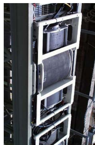
Figure 2. An XF4 and two MOD-30 projectors in a triad frame of the array. Five frames hold two MOD-30s and one XF-4. The two array-end frames hold only an XF4 each.
