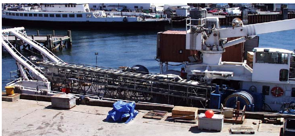
Figure 1. The Flextensional Sea Test Array installed aboard the R/V Oceanus. Its large winch is immediately forward of the long deployment rack, which occupies almost all of the stern half of the vessel. The rack protrudes 3 feet beyond the stern end to allow the array vertical section to clear the stern. The red SSC-SD amplifier milvan is shown on the 01 deck directly above the forward end of the deployment rack and the winch, both located on the vessel main deck.
