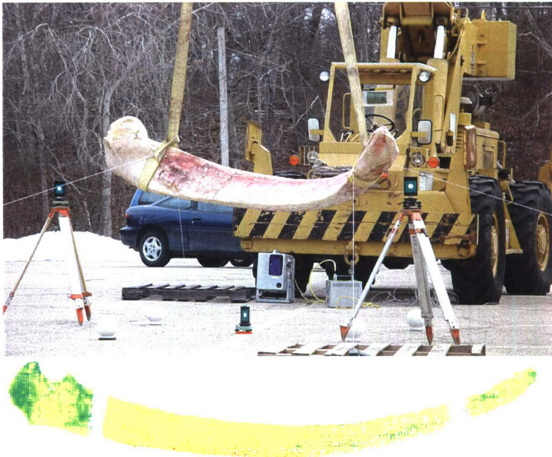
Figure 5.1: Three-dimensional laser scan of right whale mandible produces CAD-compatible point cloud detailing the external geometry of the bone. a) Above, the bone was strung from a crane such that it was free to be scanned in its entirety. b) Below, the resulting point cloud image that was transformed into a finite element mesh. In both images, the caudal end is at left, while the rostral apex is at the right. The image gaps in b designate the location of holding straps visible in a.
