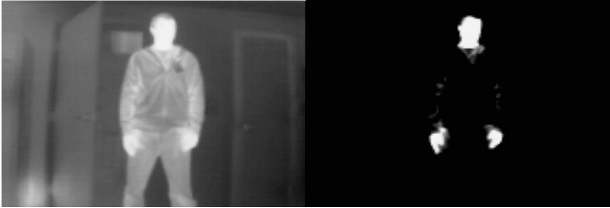
Figure 1: Thermal Imagery from the ThermoVision A10 with and without onboard contrast enhancement processing.
