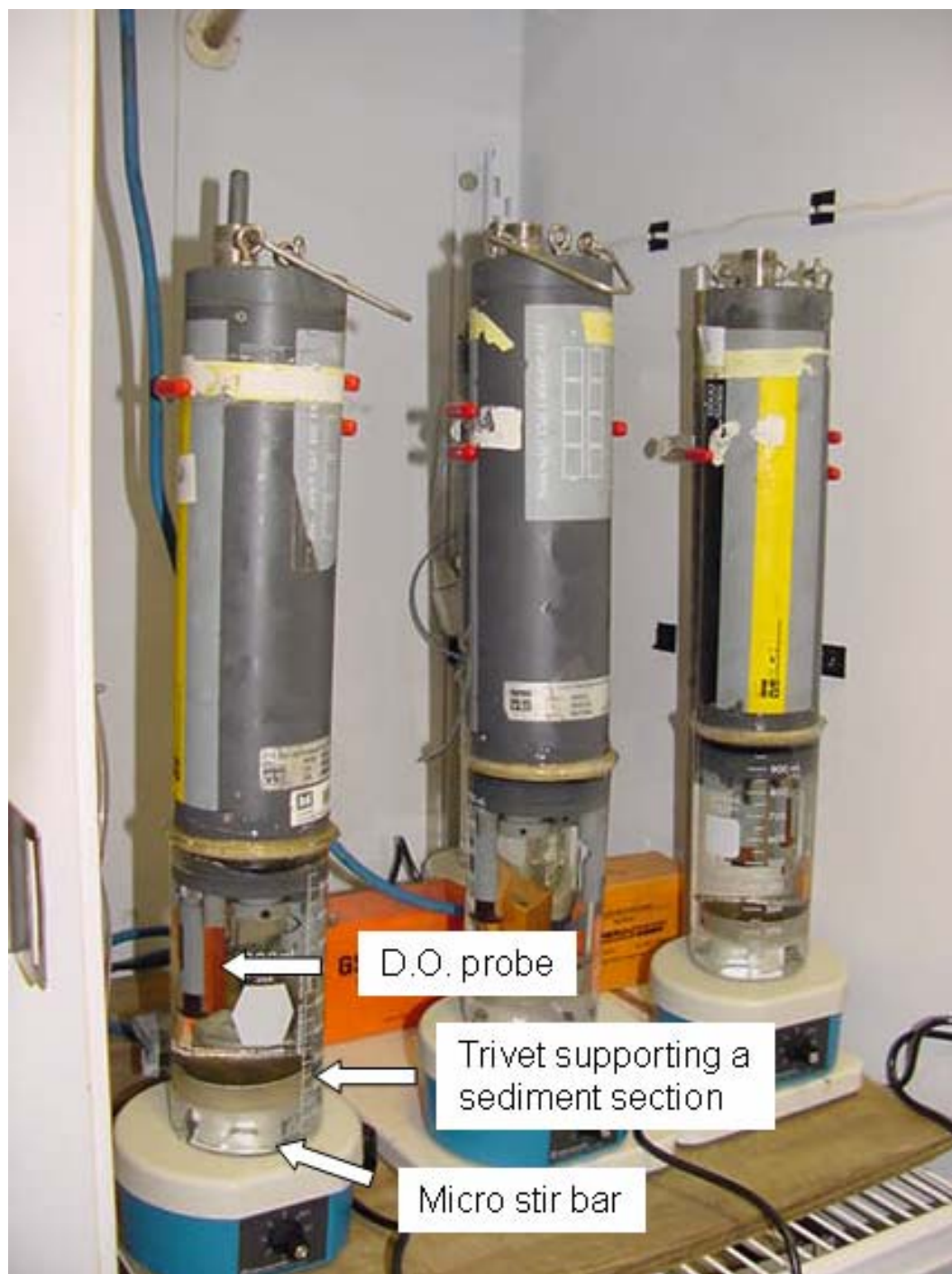
Figure 3. Methods for measuring sediment oxygen demand.
