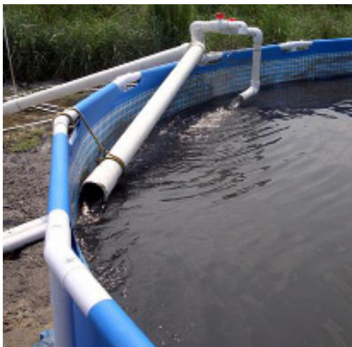
Figure 11. Pumping seed/grass mixture into circular rotation for passive seed separation.
