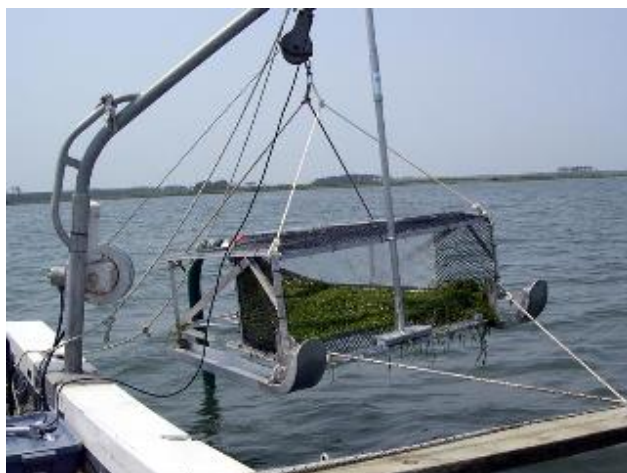
Figure 3. Harvester deployed from the side of a small vessel.
