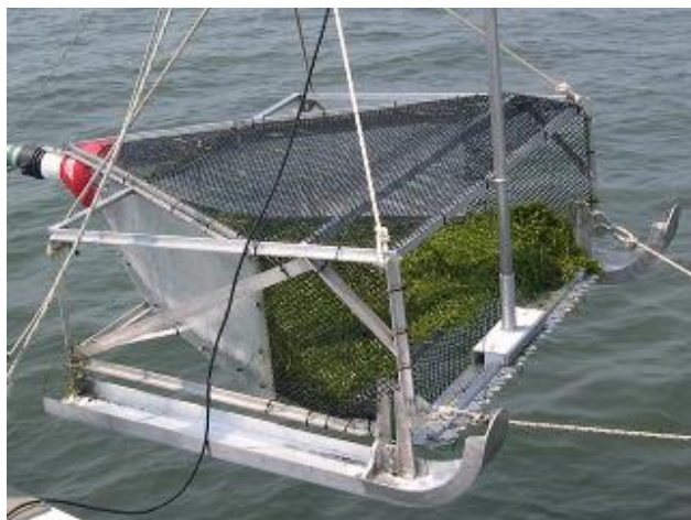
Figure 2. Modified harvester designed to be operated from a small boat.
