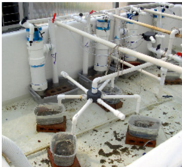
Figure 16. Circulating airlift systems used in 2005 seed storage tests.
