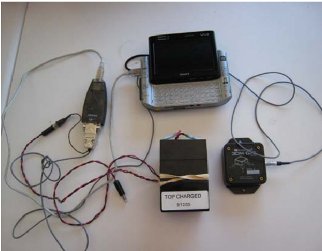
Figure 8. MARG Sensor with Peripheral Equipment for Operation.
