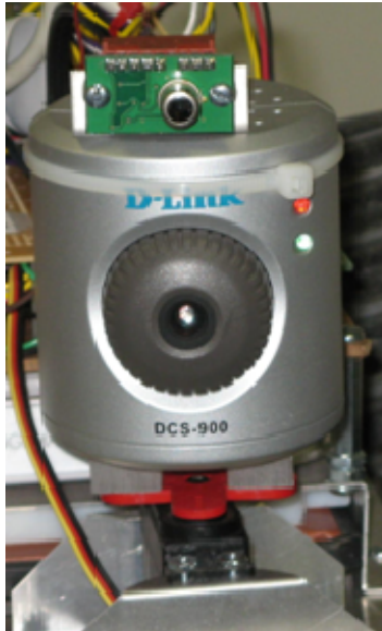
Figure 24. Camera mounted on a servo.
