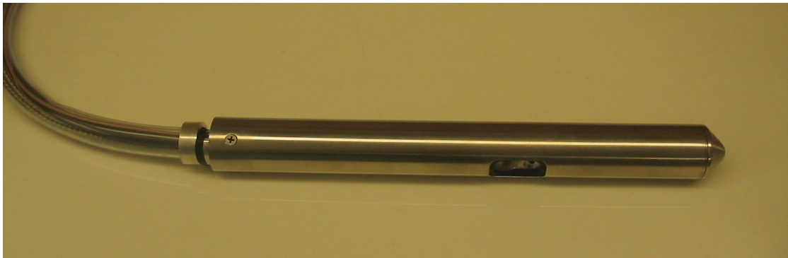
Figure 1. X-ray fluorescence spectrometer Head Unit designed to be deployed down a pre-drilled hole to analyze subsurface elements.
