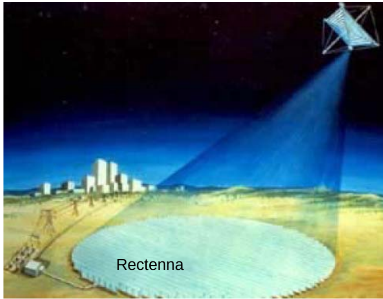
Figure 4. A Typical Ground Rectenna Illuminated by Space Solar Power Satellite (From [15]).
