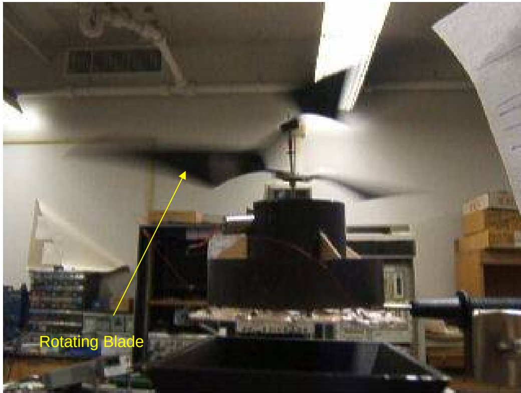
Figure 58. Rotating MAV with 4 x 4 Rectenna Array.
